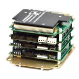
The microHydra supports up to 8 PAL/NTSC/RS-170 recording channels for capturing multiple live video cameras, RS-170 signals and FLIR. In addition, two HD-SDI inputs supporting KLV meta-data (to STANAG 4609) extraction and processing are provided to handle high-end imaging of EOIR HD
