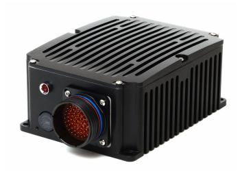
The nanoHydra-SD4 features a dedicated hardware H.264 compression engine that can encode all 4 video channels at full size and frame-rate. The flexible RTSP/RTP streaming engine supports Unicast and Multicast and streams each channel over the GigE Ethernet to client systems for low latency viewing and analysis. The nanoHydra-SD4 also supports 4 channels of audio which can be captured and streamed with the video data.
