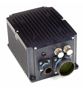
The microHydra-SD8 features a dedicated hardware H.264 compression engine that can encode all 8 video channels at full size and frame-rate. The flexible RTSP/RTP streaming engine supports Unicast and Multicast and streams each channel over the GigE Ethernet to client systems for low latency viewing and analysis. The microHyrda-SD8 also supports 4 channels of audio which can be captured and streamed with the video data.
